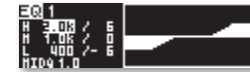
Here, we've raised the HI band by 6 dB, and lowered the LO band by the same amount
